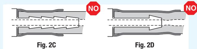
In Fig. 2C, the ferrule is much shorter than the barbed insert. Without the protection of the ferrule, repeated harsh flexing of the hose at the fitting can damage the tube. In addition, the short ferrule does not take full advantage of the sealing or retention properties of the barbed insert.
