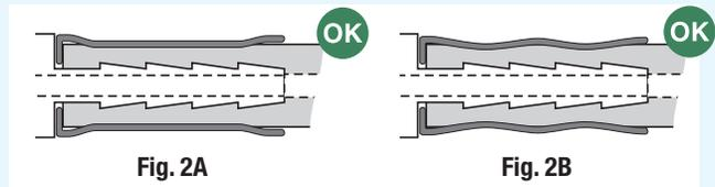
In figures 2A and 2B above, two styles of crimping die have been used successfully. The ferrules and fittings are properly matched in length.
