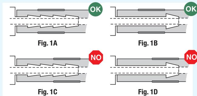
In the illustrations above, the clamps are properly positioned in Figure 1A and 1B, directly over the middle barbs and behind the first barb. This is extremely important in the case of single-barb fittings, as shown in Figure 1B, since the barb is generally much larger than the shank of the fitting. The compressed material cannot pass over the barb when under tension, thus securely holding the fitting to the hose.
