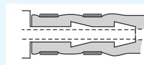
The double-barb fitting, held in place by two properly positioned clamps, provides excellent fitting retention and
