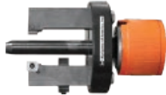
The O.D. Skiving Tool is designed with 2 cutting arms, both can be used for skiving a single hose. The advantage is that one arm can be set up to skive 4 wire hose, and the other arm can be set up to skive 6 wire hose. Simply change the insert from one tool arm, to the other and skive the appropriate hose.
