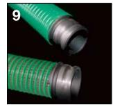
Step 9 — Insert the coupler into the hose until the hose seats against the bottom of the coupler.
