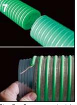
Step 7 — Screw approximately 12" of banding sleeve onto the hose; use appropriate lubricant as needed. Or, thread the banding coil between the helixes onto the hose. Slip the banding clamps onto the hose. TIP: When using banding coils, tighten clamps in a clockwise direction so the banding coil tightens down on the hose.
