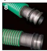
Step 8 — Insert the coupler's barbed shank into the hose, twisting counterclockwise as it enters. For ease of installation, an appropriate lubricant may be used.
