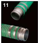
Step 11 — Install two hose clamps over the hose end above the coupling. The clamp buckles should be located 180° apart. When using banding coils, be sure to tighten clamps in a clockwise direction so the banding coils tighten down on the hose
