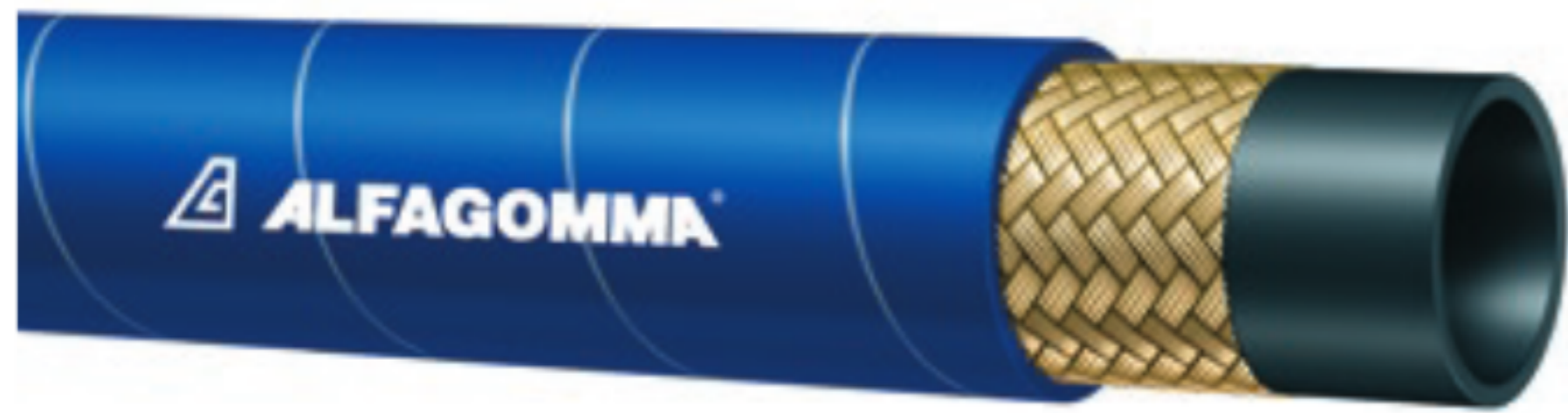
Single wire braid HIGH TEMP 1SN Meets or exceeds SAE 100R1AT - EN 853 1SN
