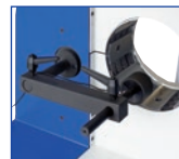
Back Limit Switch
