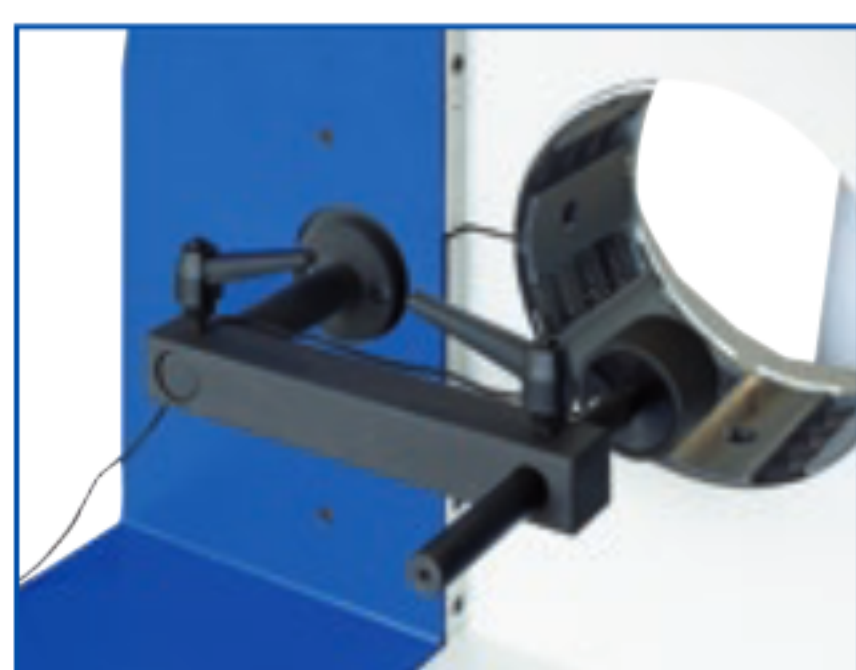
Back Limit Switch
