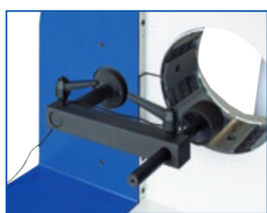
Back Limit Switch
