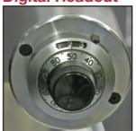
A micrometer style digital readout makes crimp set up easy and precise
