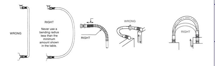
To prevent twisting and distortion, hose should be bent in the same plane as the motion of the boss to which the hose is connected.
