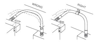
To avoid twisting in hose lines bent in two planes, clamp hose at change of plane, as shown.
