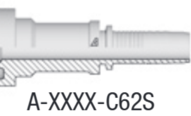
A-XXXX-C62S Other Configurations Available: A-XXXX-C624, A-XXXX-C629 Straight, 45° & 90° O-Ring Flange SAE J518 Code 62 Solid One Piece
