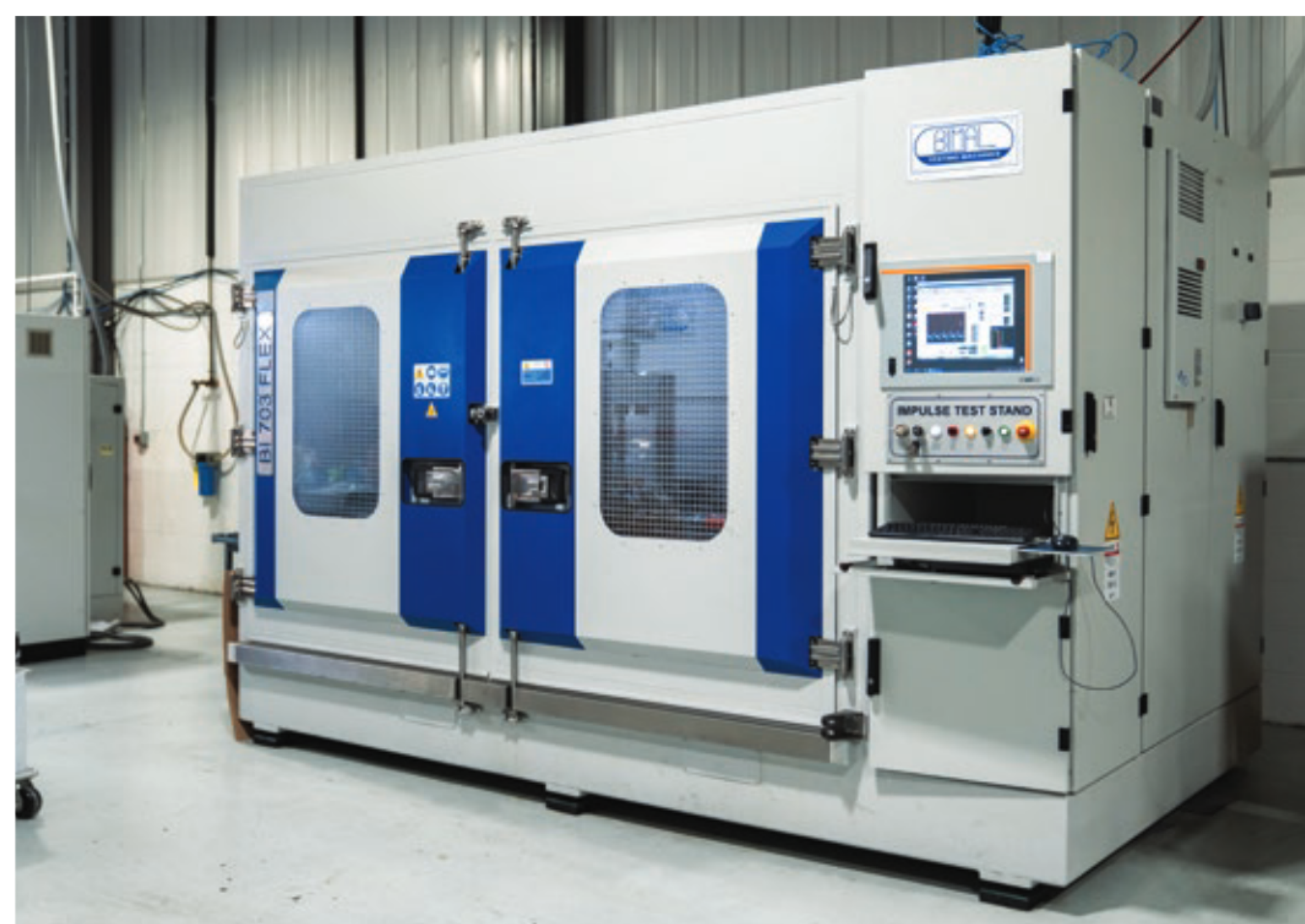
Piranhaflex hoses are rigorously tested at Piranha’s ISO 9001 quality assurance testing lab.
