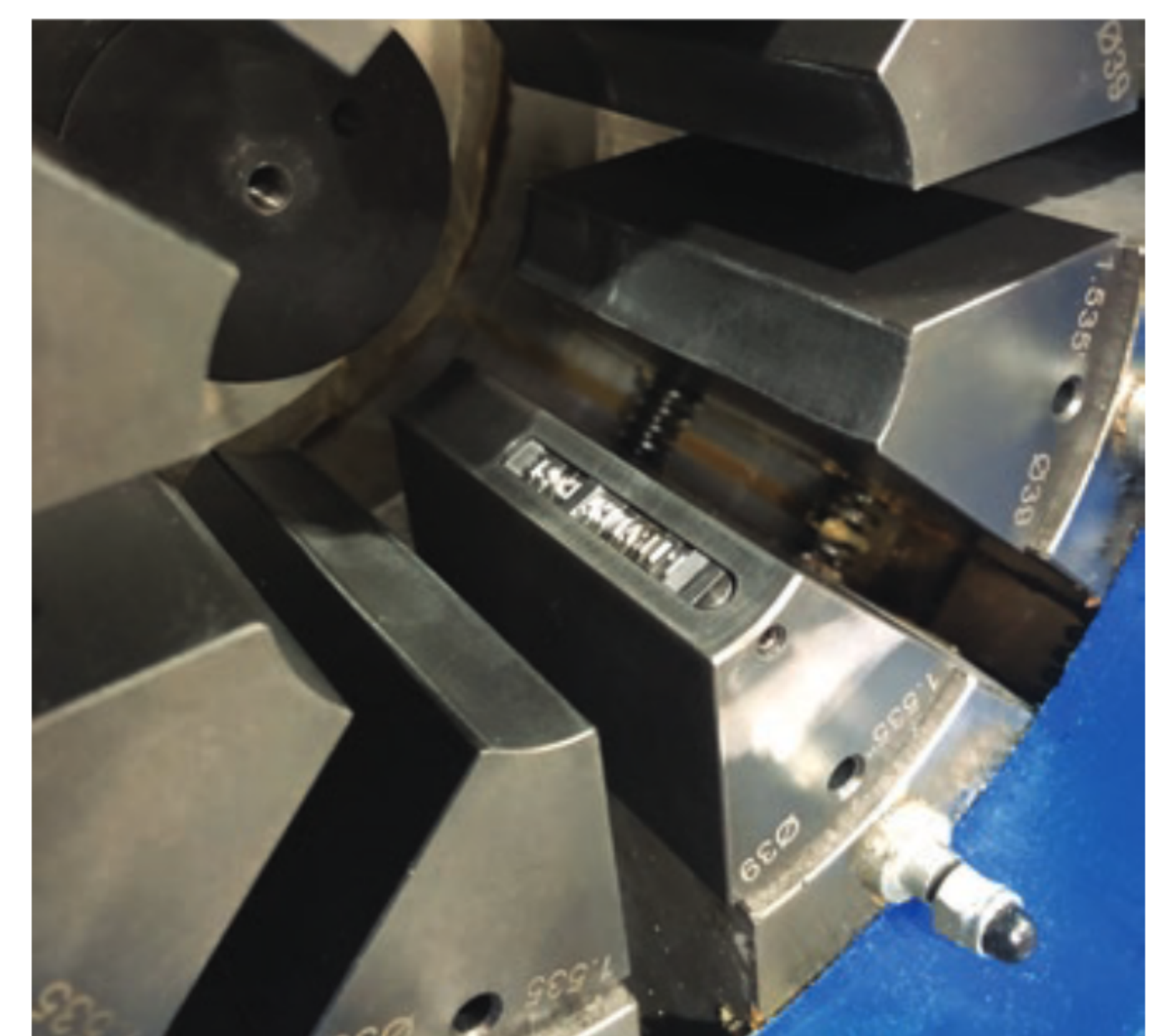
Marking Die Segments replace one of the eight standard die segments for that particular size (crimp diameter).
